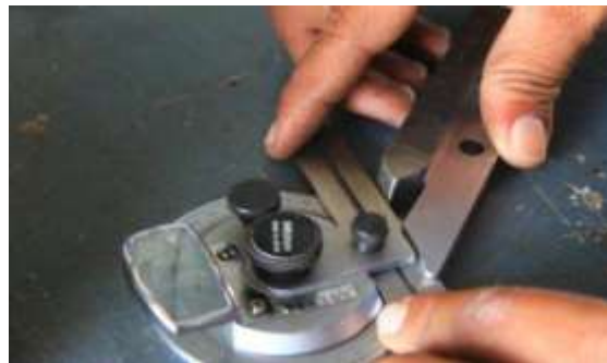
Figure 2.1.3 (b) : Measurement of tool bit angle using bevel gauge protractor.
